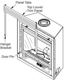
Figure 44 - Removing Top Louver Trim Panel
